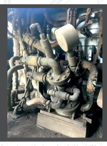
Available power up to 6 MW and 3000 Nm3/h oxygen flow, carbon and lime lances from DN32 to DN50 size. Powder injection capacity up to 150 kg/min per lance. Easy replacement of injection lances and oxygen nozzle. Only one panel opening 440 x 330 mm is sufficient for all injection functions – flame, oxygen, carbon, lime or other powder material.
